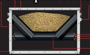
Triple seal idler arrangement separates bearings from hazardous conveyor environment
